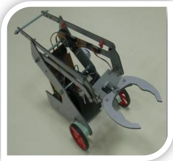
Stacker Robot operated via telephonic call developed by Students of GJIET.
