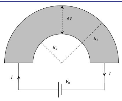
$$(A) \ \ I = \frac{V_0 t}{\pi \rho} \text{In} \left( \frac{R_2}{R_1} \right)$$
